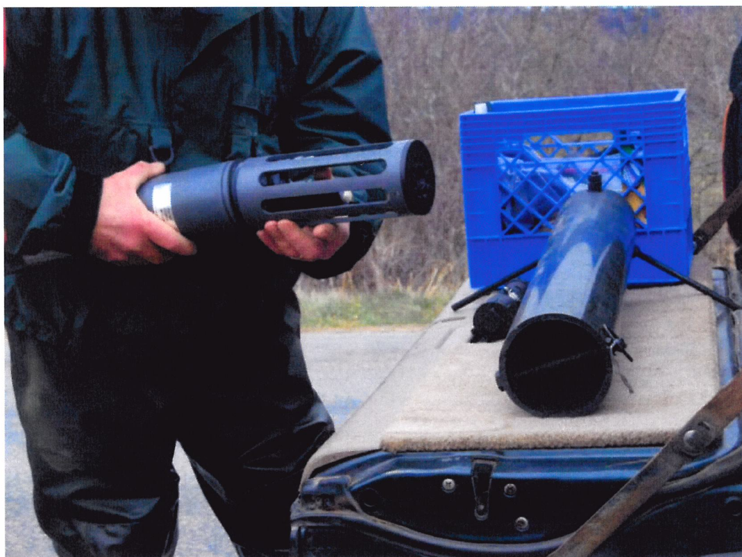
Figure 3.1 YSI Sonde and PVC tubing used for placement on River bottom.
