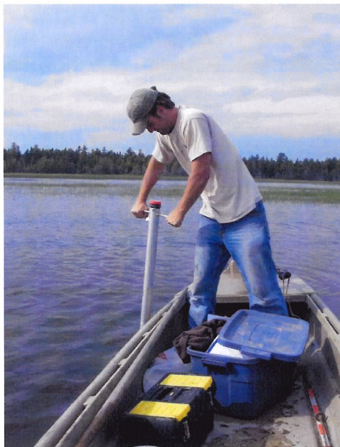
Fig. 3.2 Using a core sampler to collect sediment samples.
