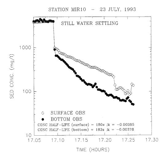
Figure 4.2.6.3-4. Relationship between sediment concentration and time during Sea Carousel settling rate measurements at post-disposal Experimental site MIR10 (Station 22).
