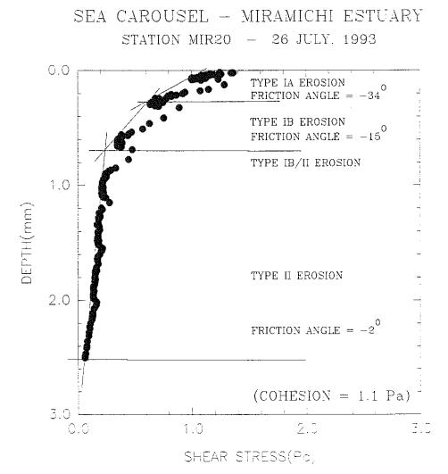
Figure 4.2.6.1-11. Relationship of shear stress and depth at post-disposal Experimental site MIR20 (Station 34).
