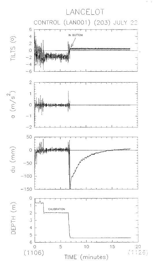
Figure 4.4-12. Calibration records for Lancelot from deployment recovery and data files (22 July 1993).
