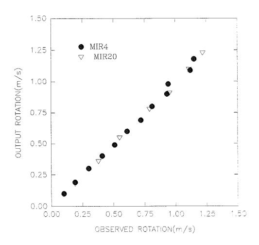
Figure 4.2.2-1. Relationship between shaft end-coder speed measurement (output) and lid rotation speed (observed).
