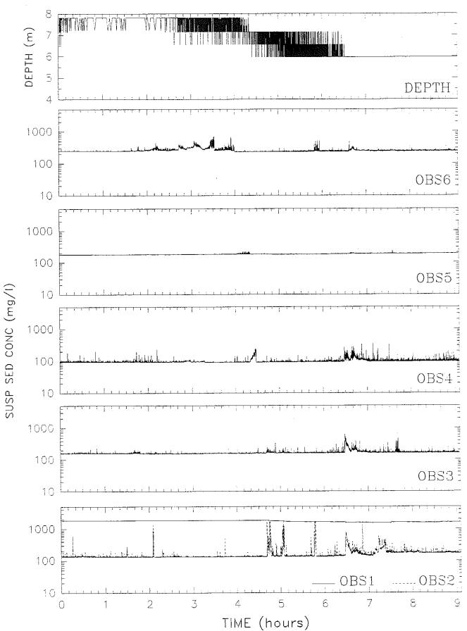
Figure 4.3.1-5. Time series of results from SOBS1 deployment at the Control site.
