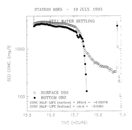
Figure 4.2.4.3-1. Relationship between sediment concentration and time during Sea Carousel settling rate measurements at Channel site MIR5 (Station 13).
