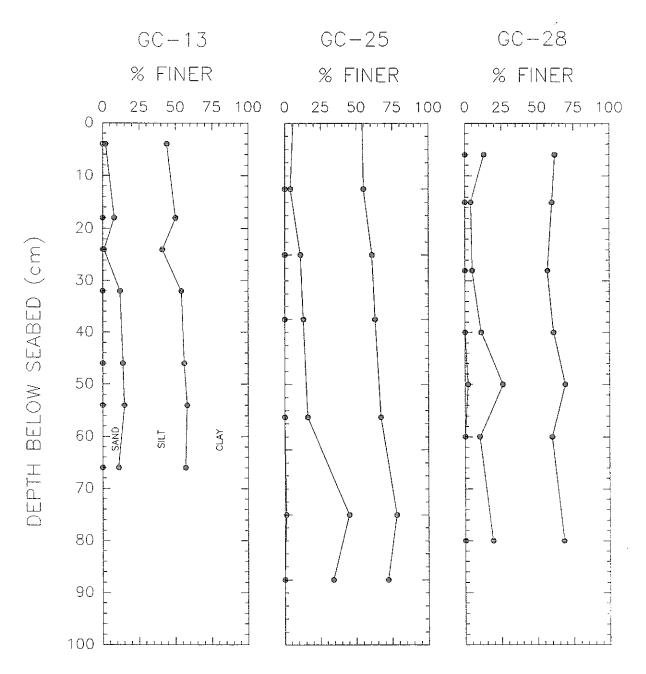
Figure 4.1-3. Variation in sediment grain size with depth for core samples taken in the Channel (GC-13), Control site (GC-25) and the post-disposal Experimental site (GC-28).
