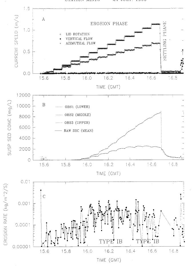
Figure 4.2.3-2. Time series of Sea Carousel results at Control site MIR13 (Station 26).
