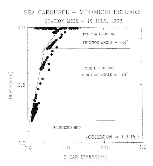
Figure 4.2.4.1-1. Relationship of shear stress and depth at Channel site MIR5 (Station 13).
