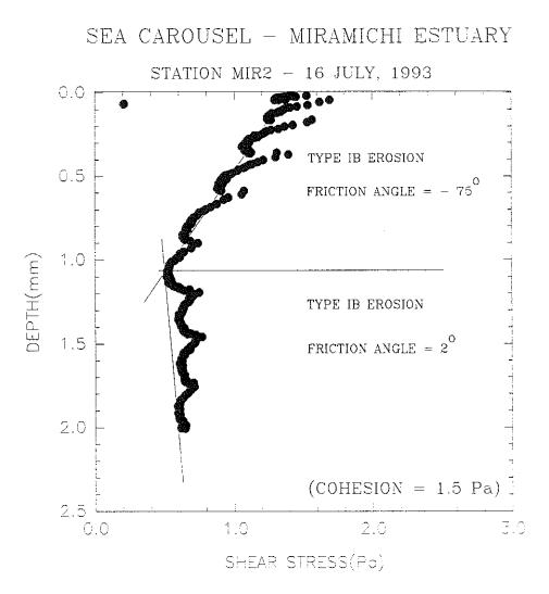
Figure 4.2.5.1-2. Relationship of shear stress and depth at pre-disposal Experimental site MIR2 (Station 7).
