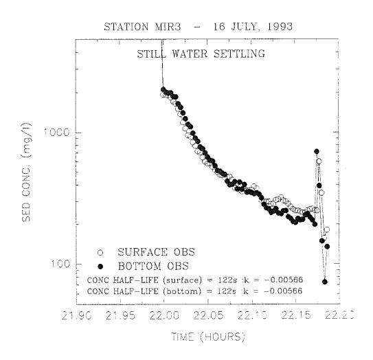
Figure 4.2.5.3-3. Relationship between sediment concentration and time during Sea Carousel settling rate measurements at pre-disposal Experimental site MIR3 (Station 8).
