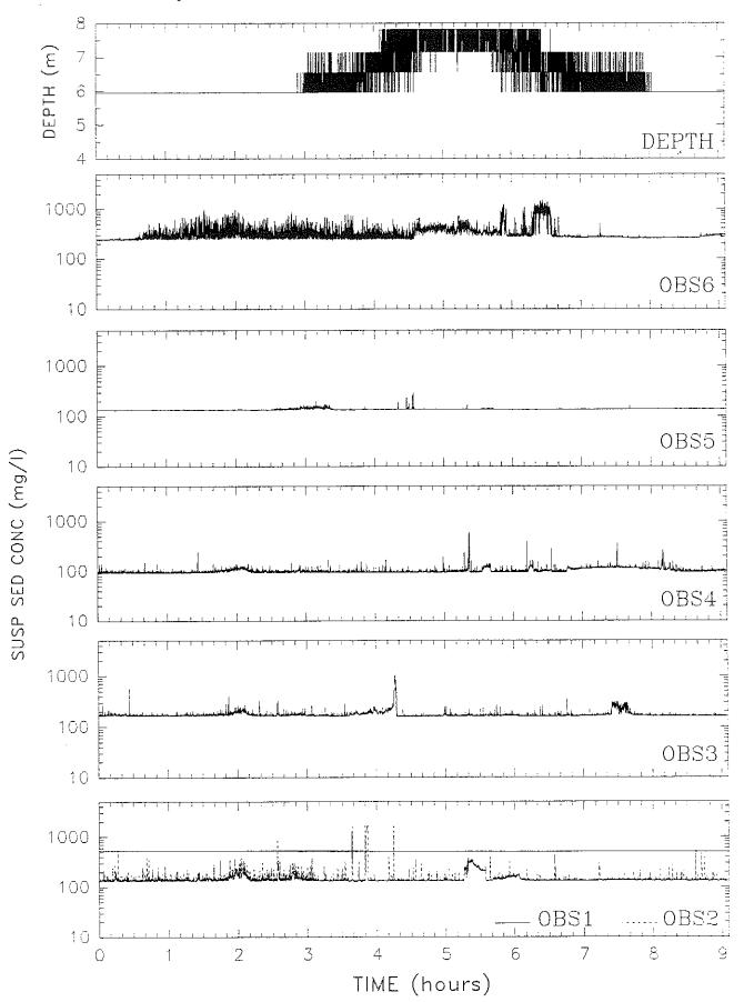
Figure 4.3.2-5. Time series of results from SOBS2 deployment at the Experimental site.
