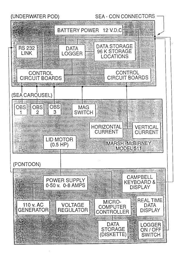
Figure 3.2-2. Schematic diagram of the configuration of the Sea Carousel.
