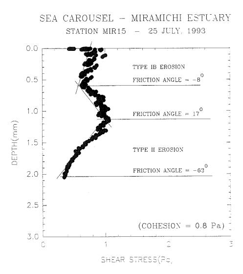
Figure 4.2.6.1-6. Relationship of shear stress and depth at post-disposal Experimental site MIR15 (Station 28).
