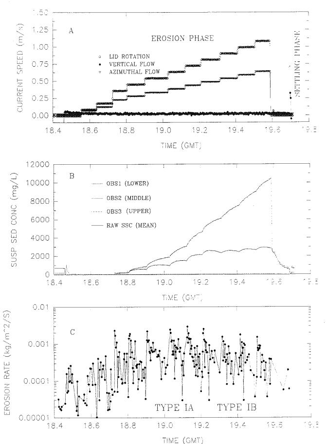
Figure 4.2.5-2. Time series of Sea Carousel results at pre-disposal Experimental site MIR2 (Station 7).
