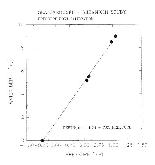
Figure 4.2.2-2. Relationship between pressure sensor measurement and water depth.
