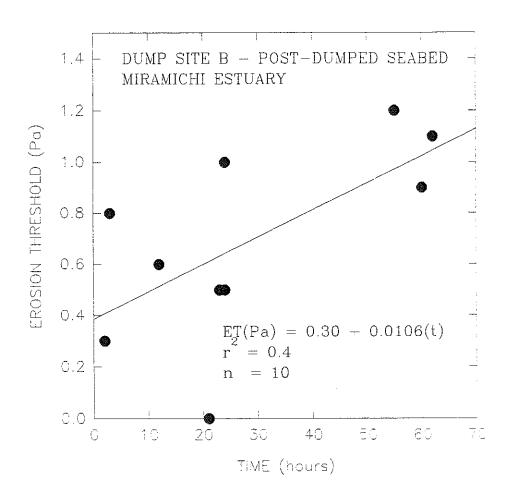
Figure 4.2.6.1-12. Time series of the erosion threshold of spoils deposited at the Experimental disposal-site.
