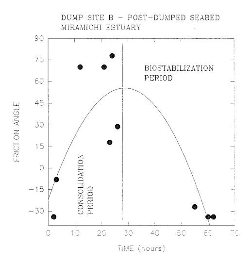
Figure 4.2.6.1-13. Time series of the near-surface friction angle at the post-disposal Experimental site.
