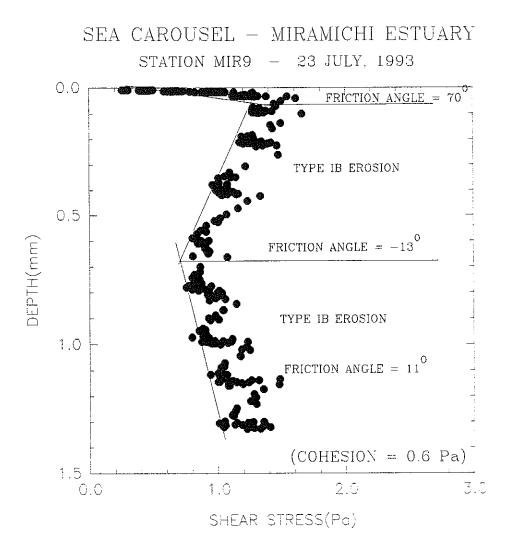
Figure 4.2.6.1-3. Relationship of shear stress and depth at post-disposal Experimental site MIR9 (Station 21).
