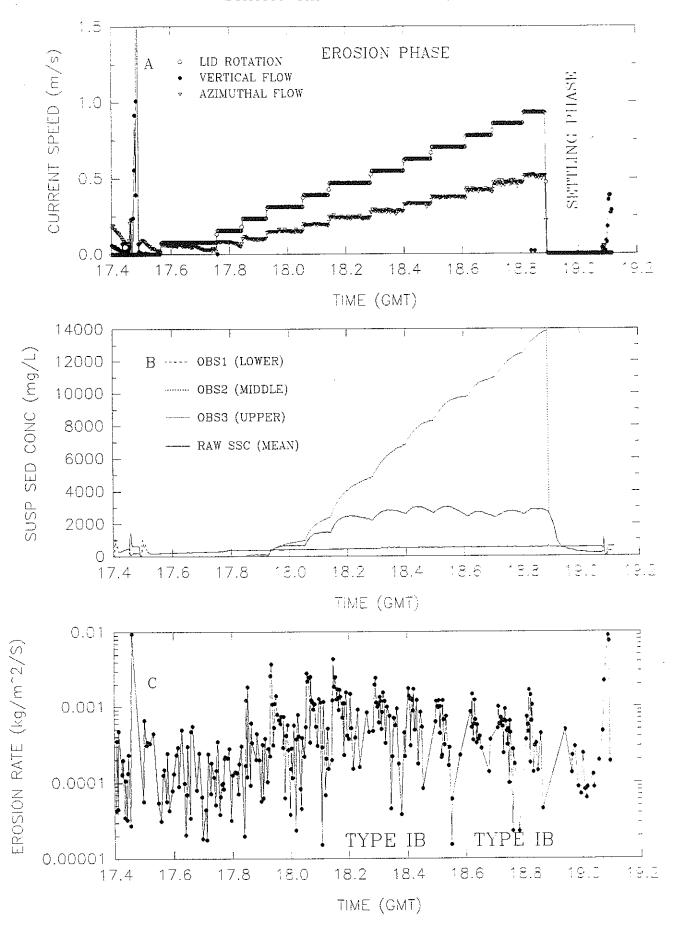
Figure 4.2.4-2. Time series of Sea Carousel results at Channel site MIR6 (Station 12).
