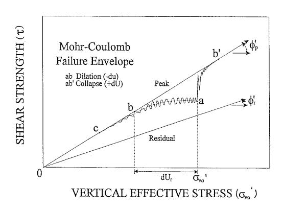
Figure 3.4-1. Relationship between shear strength and vertical effective stress.
