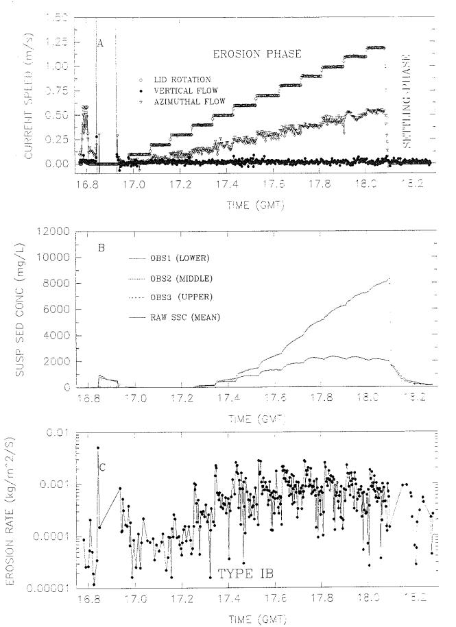
Figure 4.2.5-4. Time series of Sea Carousel results at pre-disposal Experimental site MIR3 (Station 9).
