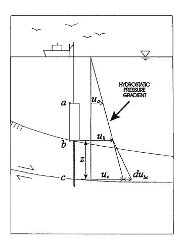
Figure 3.4.1-2. Diagram of Lancelot in the deployed configuration.
