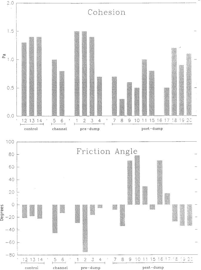
Figure 5.2-1. Trends in erosion threshold (cohesion) and friction angle.
