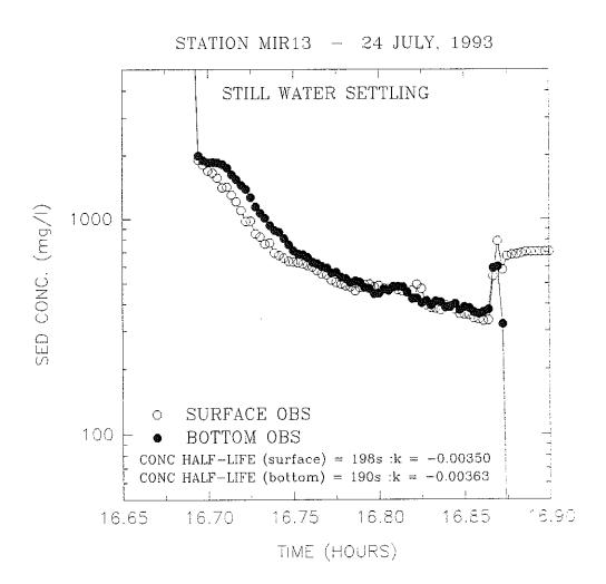
Figure 4.2.3.3-2. Relationship between sediment concentration and time during Sea Carousel settling rate measurements at Control site MIR13 (Station 26).
