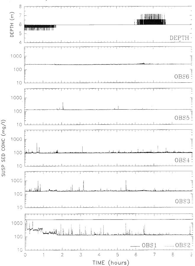
Figure 4.3.2-9. Time series of results from SOBS2 deployment at the Experimental site.
