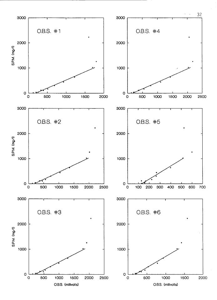
Figure 3.3-2. Calibration curves for SOBS Optical Backscatter Sensors.
