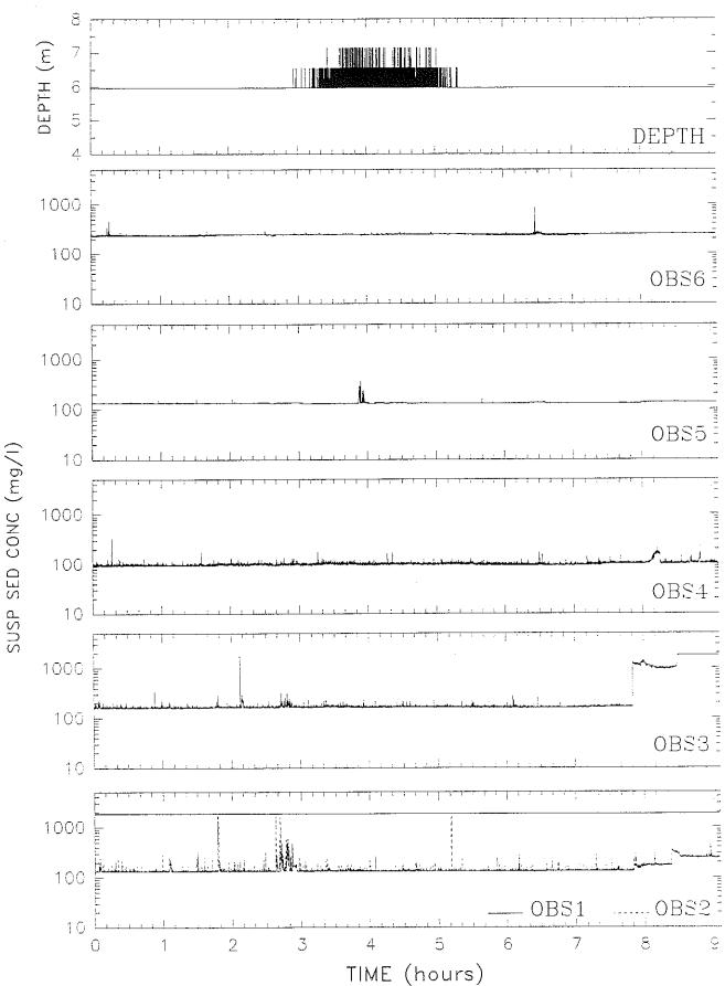
Figure 4.3.2-12. Time series of results from SOBS2 deployment at the Experimental site.
