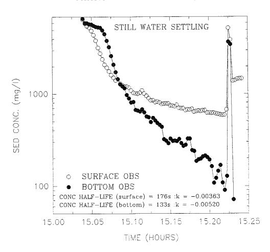
Figure 4.2.6.3-8. Relationship between sediment concentration and time during Sea Carousel settling rate measurements at post-disposal Experimental site MIR18 (Station 32).
