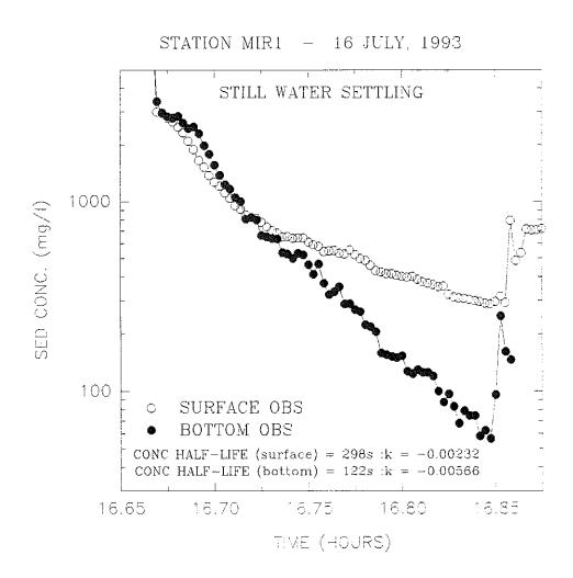
Figure 4.2.5.3-1. Relationship between sediment concentration and time during Sea Carousel settling rate measurements at pre-disposal Experimental site MIR1 (Station 6).
