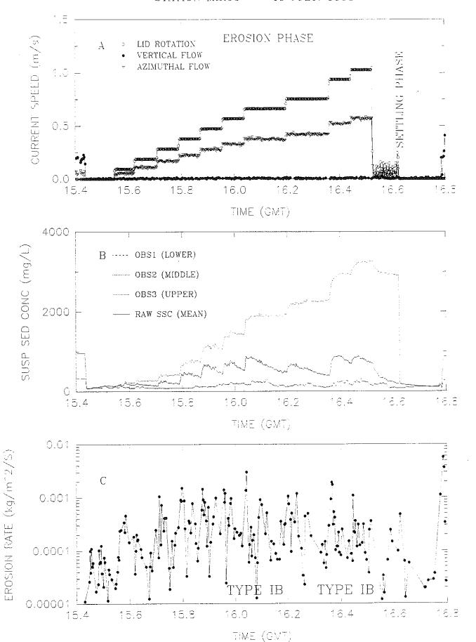
Figure 4.2.6-7. Time series of Sea Carousel results at post-disposal Experimental site MIR16 (Station 29).
