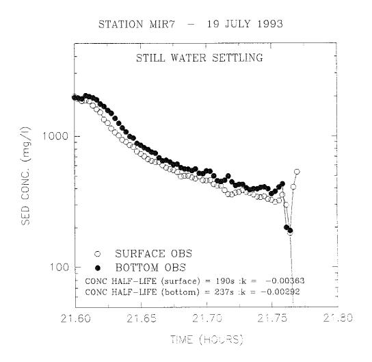
Figure 4.2.6.3-1. Relationship between sediment concentration and time during Sea Carousel settling rate measurements at post-disposal Experimental site MIR7 (Station 8).
