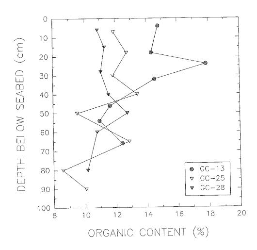
Figure 4.1-1. Variation in sediment organic content with depth for core samples taken in the Channel (GC-13), Control site (GC-25) and the post-disposal Experimental site (GC-28).
