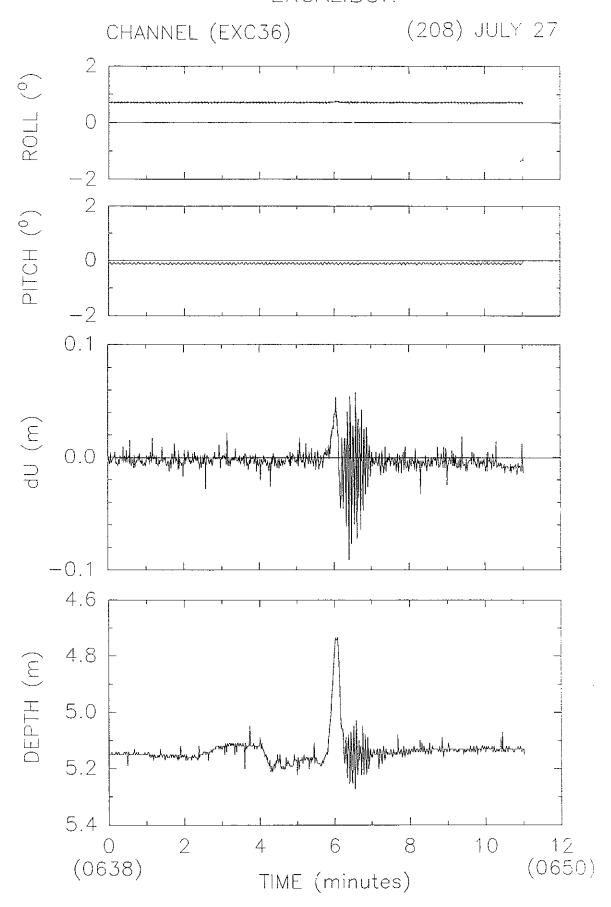
Figure 4.4-14. Excalibur results during passage (outgoing) of the Hubert Tanthier (27 July 1993) at the Channel site.
