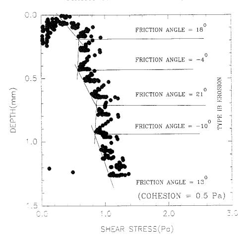
Figure 4.2.6.1-8. Relationship of shear stress and depth at post-disposal Experimental site MIR17 (Station 30).
