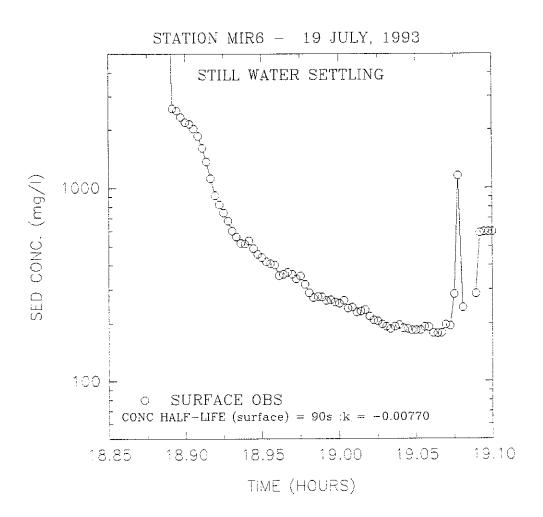
Figure 4.2.4.3-2. Relationship between sediment concentration and time during Sea Carousel settling rate measurements at Channel site MIR6 (Station 12).
