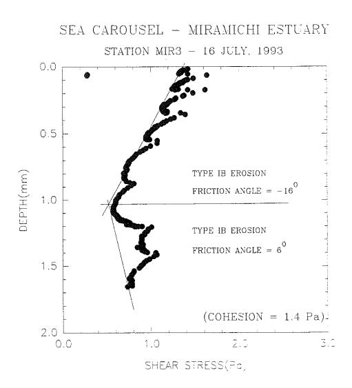
Figure 4.2.5.1-3. Relationship of shear stress and depth at pre-disposal Experimental site MIR3 (Station 8).
