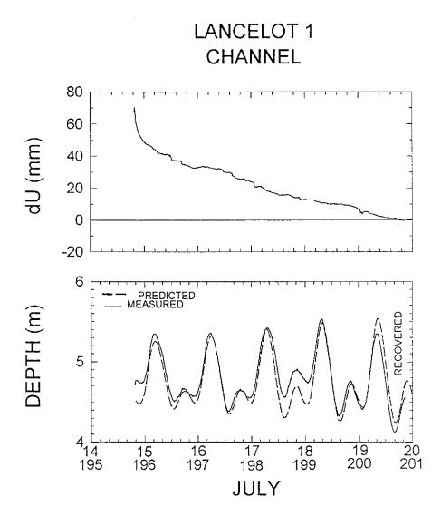
Figure 4.4-1. Pore pressure decay curve for Lancelot 1 deployment at the Channel site (Station 4).
