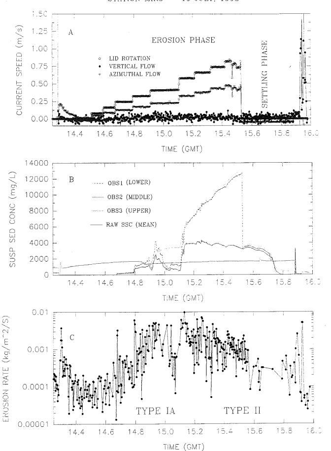
Figure 4.2.4-1. Time series of Sea Carousel results at Channel site MIR5 (Station 13).
