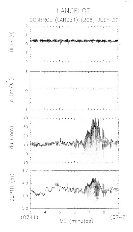
Figure 4.4-9. Expanded view of Lancelot results during passage (outgoing) of the Hubert Tanthier (27 July 1993) at the Control site.
