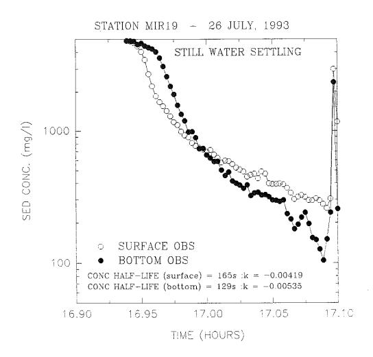
Figure 4.2.6.3-9. Relationship between sediment concentration and time during Sea Carousel settling rate measurements at post-disposal Experimental site MIR19 (Station 33).
