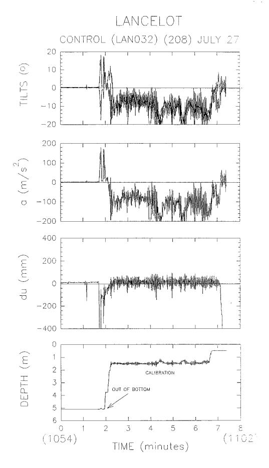
Figure 4.4-13. Calibration records for Lancelot from deployment recovery and data files (27 July 1993).
