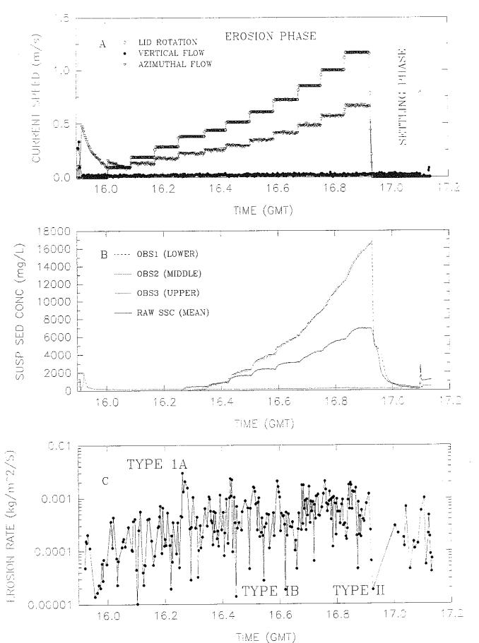
Figure 4.2.6-10. Time series of Sea Carousel results at post-disposal Experimental site MIR19 (Station 33).
