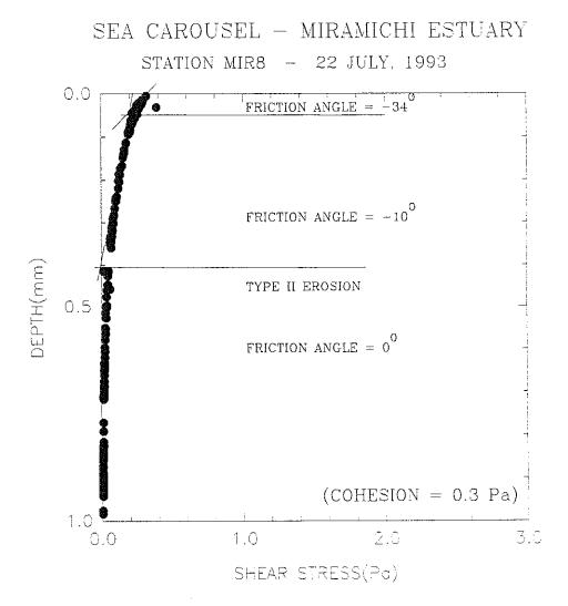
**Figure 4.2.6.1-2.** Relationship of shear stress and depth at post-disposal Experimental site MIR8 (Station 20).
