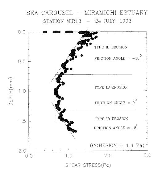
Figure 4.2.3.1-2. Relationship of shear stress and depth at Control site MIR13 (Station 26).
