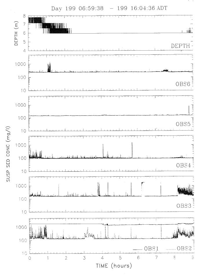
Figure 4.3.1-11. Time series of results from SOBS1 deployment at the Control site.
