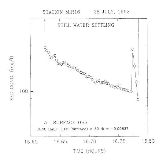
Figure 4.2.6.3-6. Relationship between sediment concentration and time during Sea Carousel settling rate measurements at post-disposal Experimental site MIR16 (Station 29).
