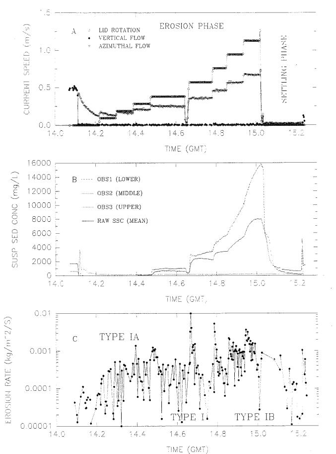
Figure 4.2.6-9. Time series of Sea Carousel results at post-disposal Experimental site MIR18 (Station 32).
