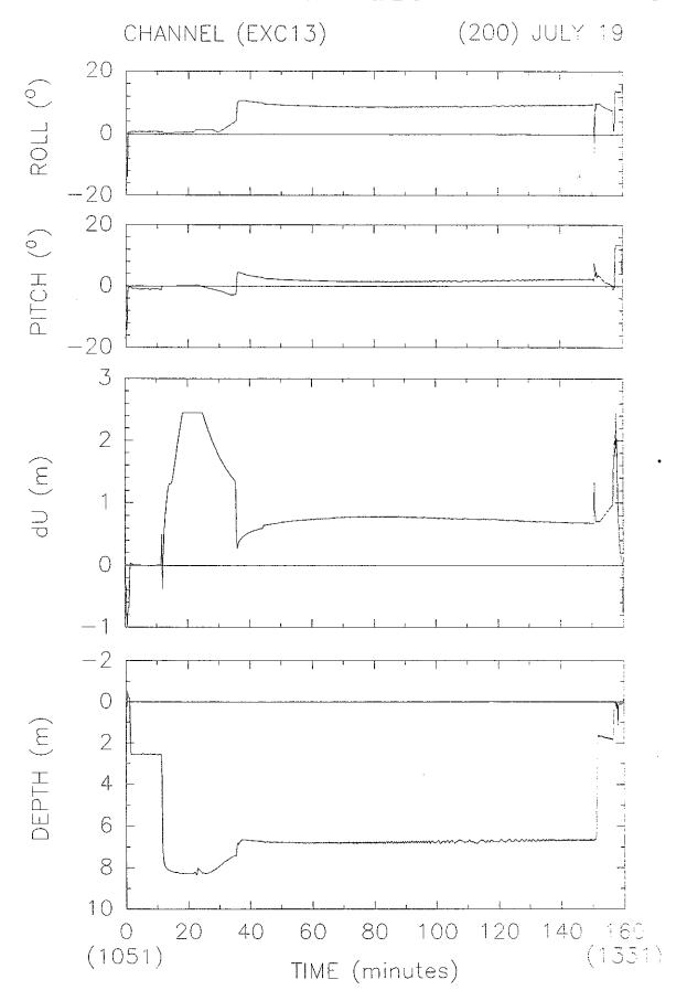
Figure 4.5-3. Time series results for Excalibur deployment at Channel site (Station 13).
