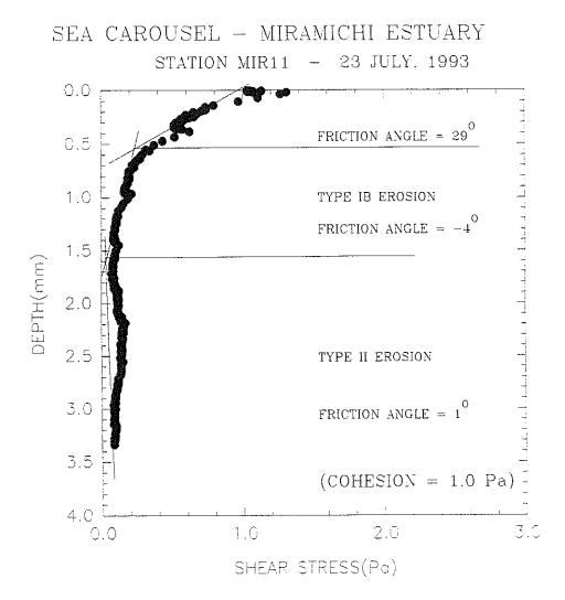
Figure 4.2.6.1-5. Relationship of shear stress and depth at post-disposal Experimental site MIR11 (Station 23).
