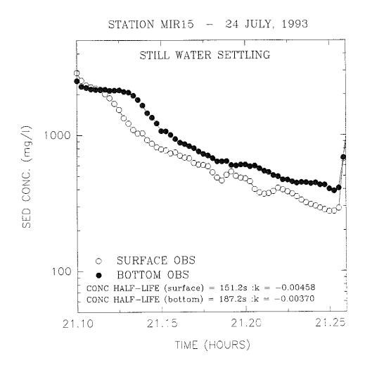
Figure 4.2.6.3-5. Relationship between sediment concentration and time during Sea Carousel settling rate measurements at post-disposal Experimental site MIR15 (Station 28).
