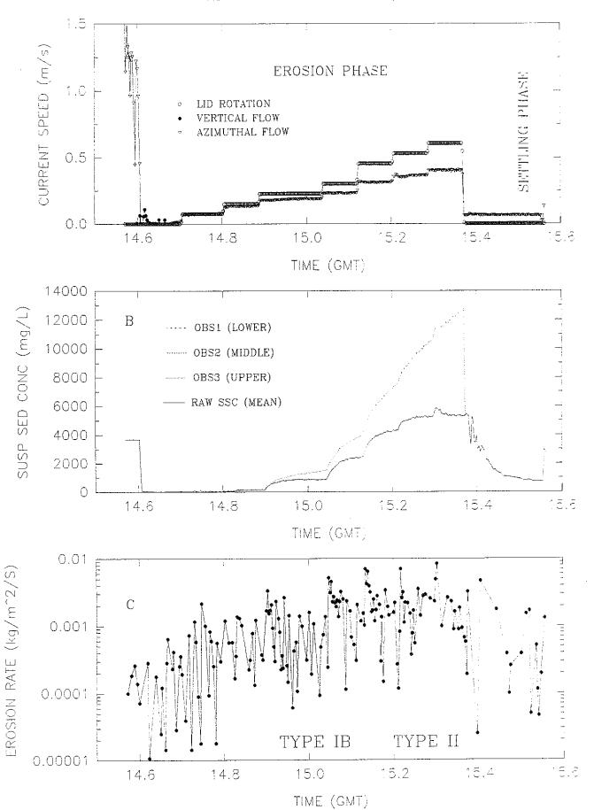
Figure 4.2.6-2. Time series of Sea Carousel results at post-disposal Experimental site MIR8 (Station 20).
