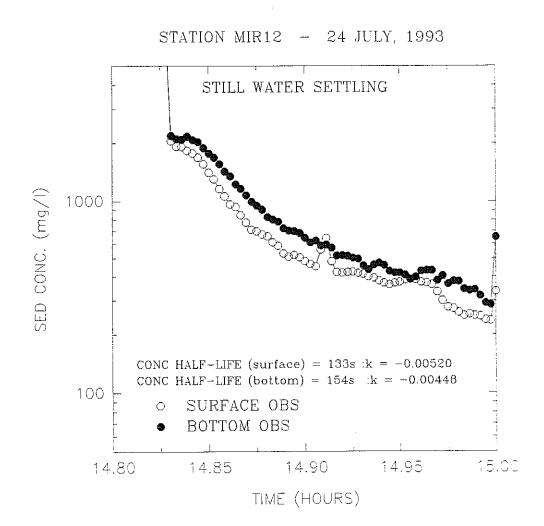
Figure 4.2.3.3-1. Relationship between sediment concentration and time during Sea Carousel settling rate measurements at Control site MIR12 (Station 25).
