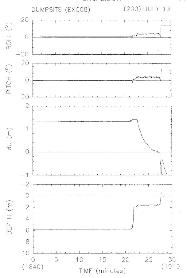
Figure 4.5-8. Time series results for Excalibur deployment at Experimental site (Station 8).
