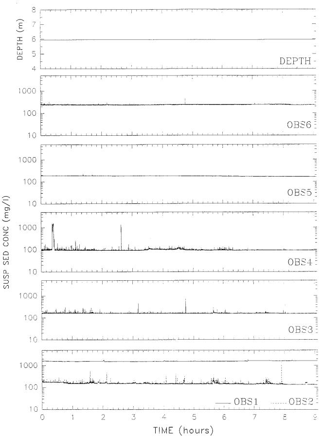
Figure 4.3.1-6. Time series of results from SOBS1 deployment at the Control site.
