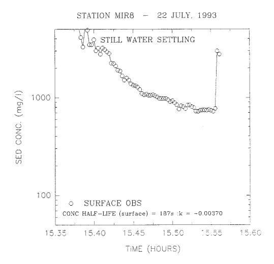
Figure 4.2.6.3-2. Relationship between sediment concentration and time during Sea Carousel settling rate measurements at post-disposal Experimental site MIR8 (Station 20).
