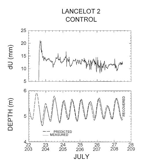
Figure 4.4-2. Pore pressure decay curve for Lancelot 2 deployment at the Control site (Station 18).
