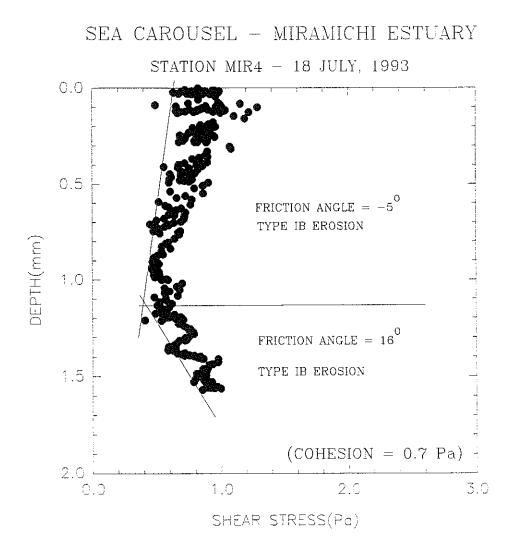
Figure 4.2.5.1-4. Relationship of shear stress and depth at pre-disposal Experimental site MIR4 (Station 9).
