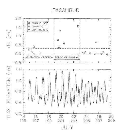
Figure 4.5-19. Time series of Excalibur residual excess pore pressures for all sites in relationship to time frame for disposal activities.
