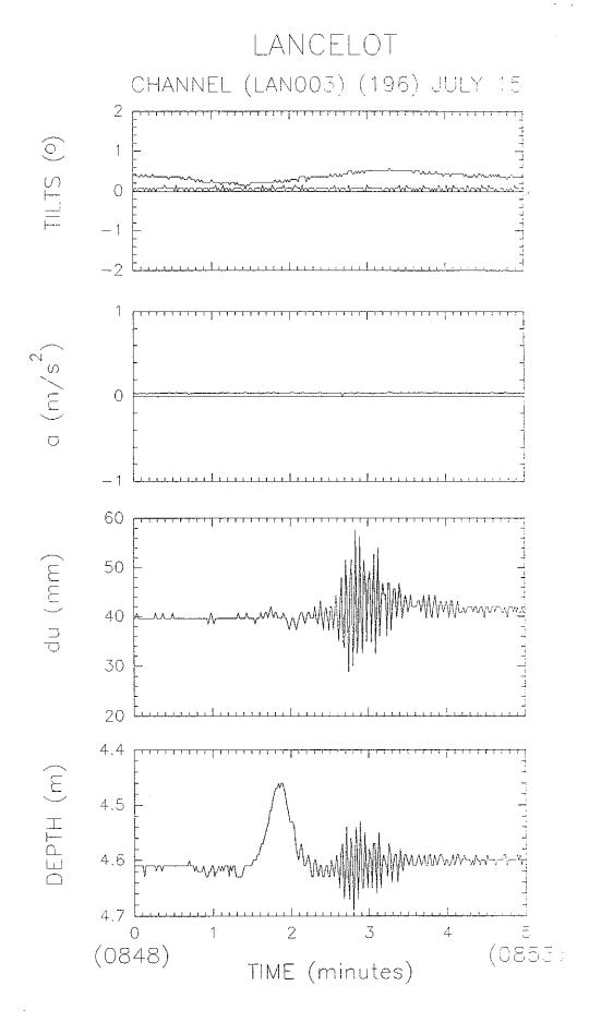
Figure 4.4-4. Lancelot results during passage (incoming) of the M/V Mariner (15 July 1993) at the Channel site.
