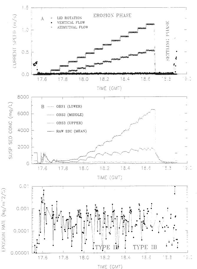
Figure 4.2.6-8. Time series of Sea Carousel results at post-disposal Experimental site MIR17 (Station 30).
