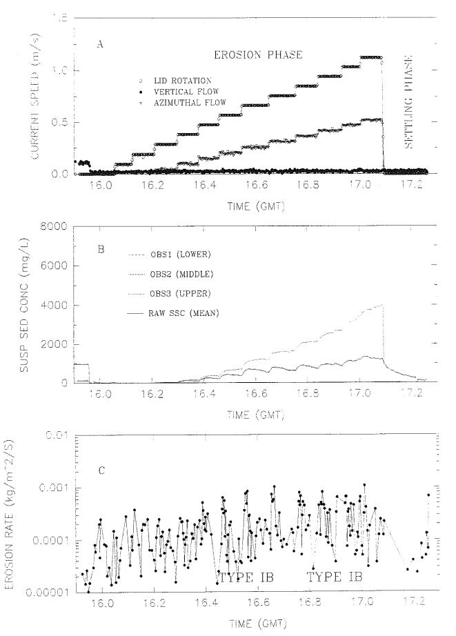
Figure 4.2.6-4. Time series of Sea Carousel results at post-disposal Experimental site MIR10 (Station 22).
