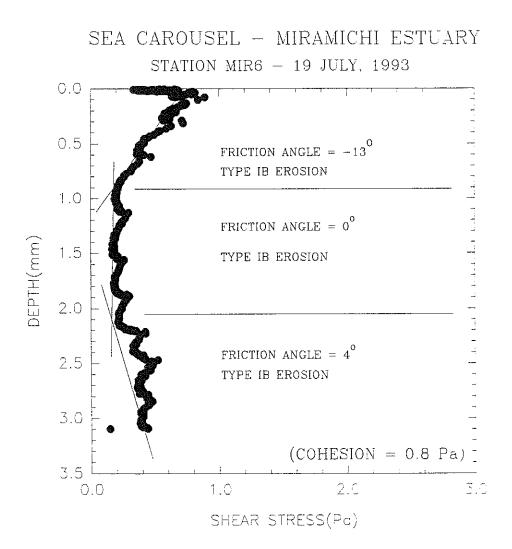
Figure 4.2.4.1-2. Relationship of shear stress and depth at Channel site MIR6 (Station 12).
