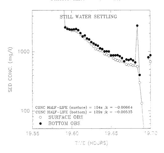
Figure 4.2.5.3-2. Relationship between sediment concentration and time during Sea Carousel settling rate measurements at pre-disposal Experimental site MIR2 (Station 7).
