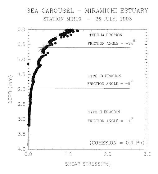
Figure 4.2.6.1-10. Relationship of shear stress and depth at post-disposal Experimental site MIR19 (Station 33).
