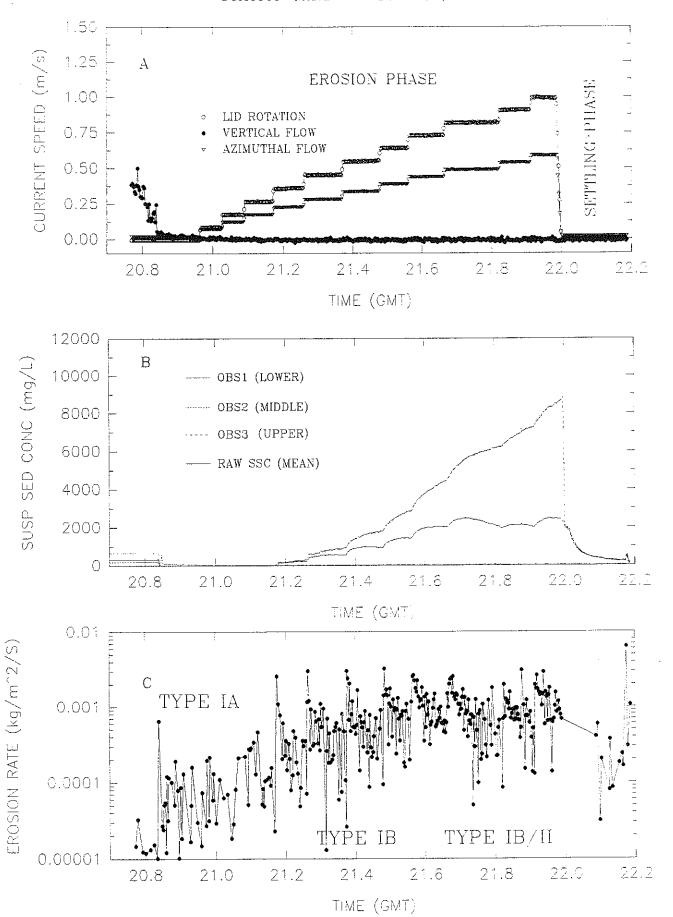
Figure 4.2.5-3. Time series of Sea Carousel results at pre-disposal Experimental site MIR3 (Station 8).
