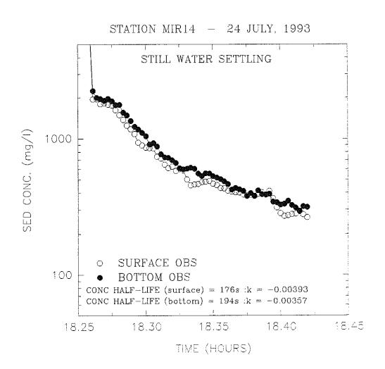
Figure 4.2.3.3-3. Relationship between sediment concentration and time during Sea Carousel settling rate measurements at Control site MIR14 (Station 27).
