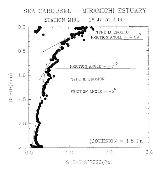
Figure 4.2.5.1-1. Relationship of shear stress and depth at pre-disposal Experimental site MIR1 (Station 6).
