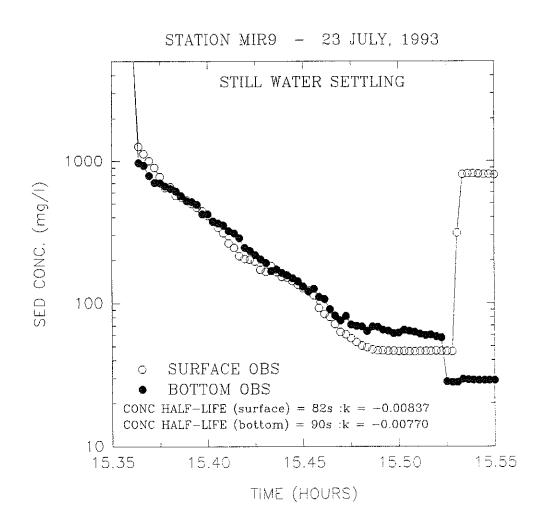
Figure 4.2.6.3-3. Relationship between sediment concentration and time during Sea Carousel settling rate measurements at post-disposal Experimental site MIR9 (Station 21).
