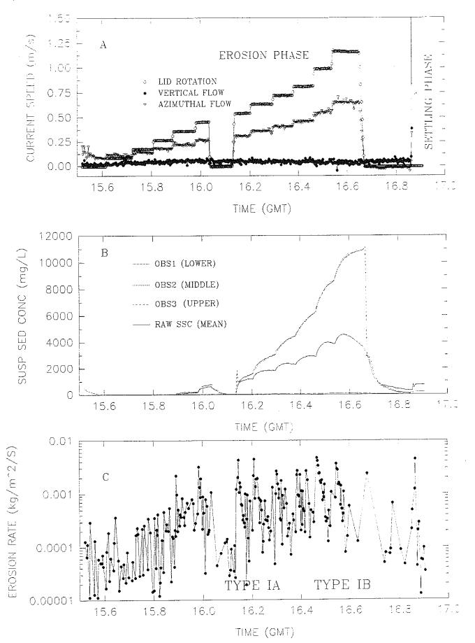
Figure 4.2.5-1. Time series of Sea Carousel results at pre-disposal Experimental site MIR1 (Station 6).
