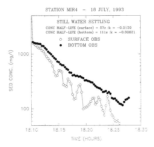
Figure 4.2.5.3-4. Relationship between sediment concentration and time during Sea Carousel settling rate measurements at pre-disposal Experimental site MIR4 (Station 9).
