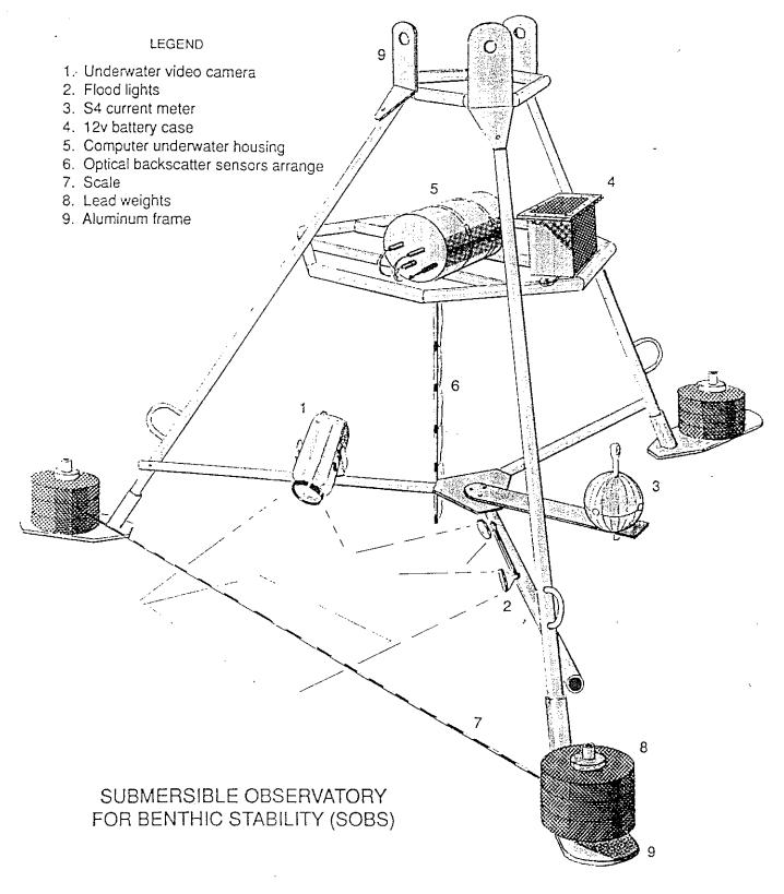
Figure 3.3-1. The SOBS system (note that the current meter was not installed during this study).
