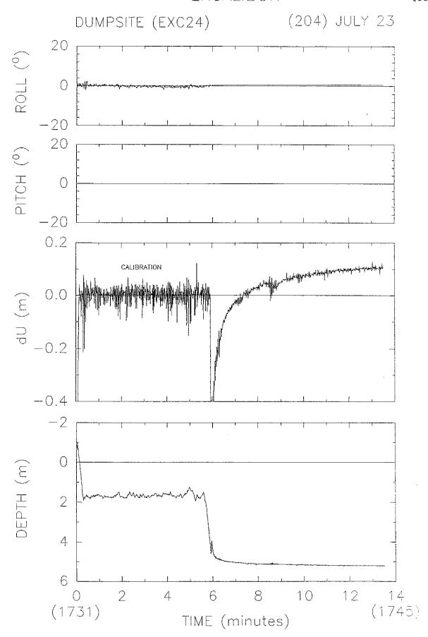
Figure 4.5-13. Time series results for Excalibur deployment at Experimental site (Station 24).
