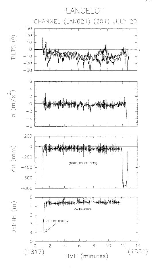
Figure 4.4-11. Calibration records for Lancelot from deployment recovery and data files (20 July 1993).
