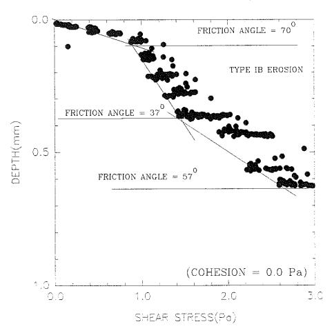
Figure 4.2.6.1-7. Relationship of shear stress and depth at post-disposal Experimental site MIR16 (Station 29).
