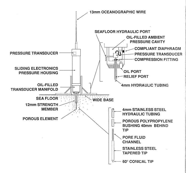
Figure 3.4.1-1. Schematic diagram of Lancelot.
