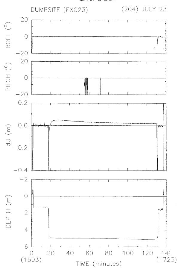
Figure 4.5-12. Time series results for Excalibur deployment at Experimental site (Station 23).
