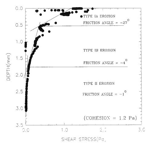
Figure 4.2.6.1-9. Relationship of shear stress and depth at post-disposal Experimental site MIR18 (Station 32).
