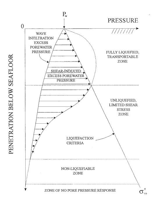
Figure 3.4-2. Diagram illustrating how waves can cause internal shearing and lead to the destabilization of sediment structure.
