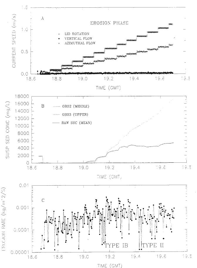
Figure 4.2.6-5. Time series of Sea Carousel results at post-disposal Experimental site MIR11 (Station 23).
