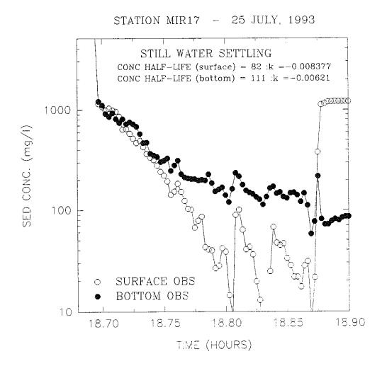
Figure 4.2.6.3-7. Relationship between sediment concentration and time during Sea Carousel settling rate measurements at post-disposal Experimental site MIR17 (Station 30).
