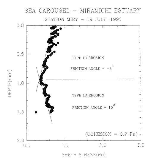
Figure 4.2.6.1-1. Relationship of shear stress and depth at post-disposal Experimental site MIR7 (Station 8).
