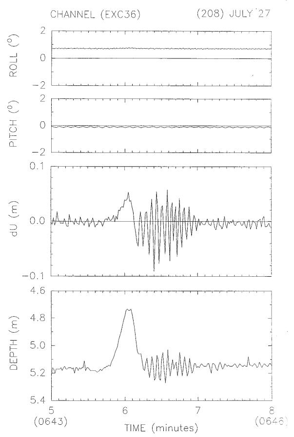
Figure 4.4-15. Expanded view of Excalibur results during passage (outgoing) of the Hubert Tanthier (27 July 1993) at the Channel site.
