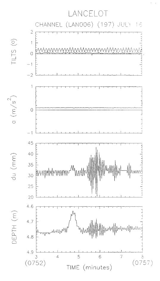
Figure 4.4-6. Expanded view of Lancelot results during passage (outgoing) of the M/V Mariner (16 July 1993) at the Channel site.
