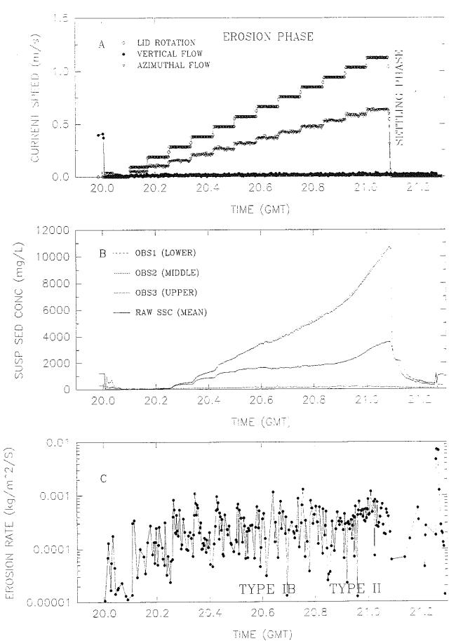
Figure 4.2.6-6. Time series of Sea Carousel results at post-disposal Experimental site MIR15 (Station 28).
