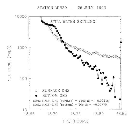
Figure 4.2.6.3-10. Relationship between sediment concentration and time during Sea Carousel settling rate measurements at post-disposal Experimental site MIR20 (Station 34).
