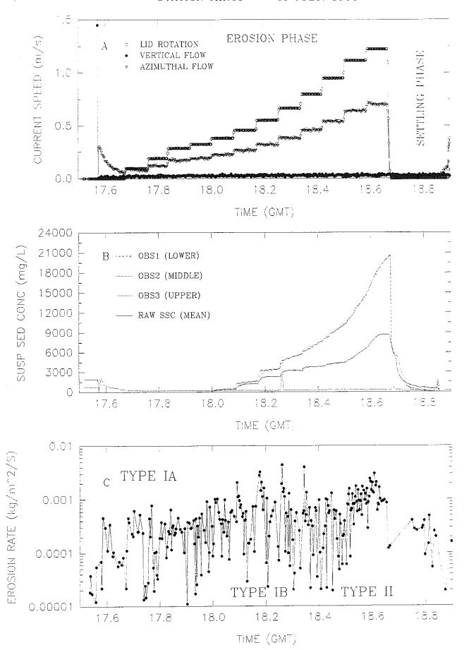
Figure 4.2.6-11. Time series of Sea Carousel results at post-disposal Experimental site MIR20 (Station 34).
